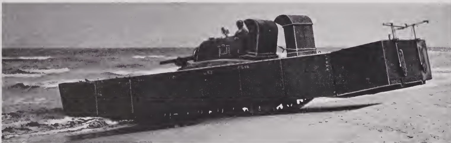
FIGURE 24. M-4 M1 medium tank equipped with Ritchie T-6 flotation device.
